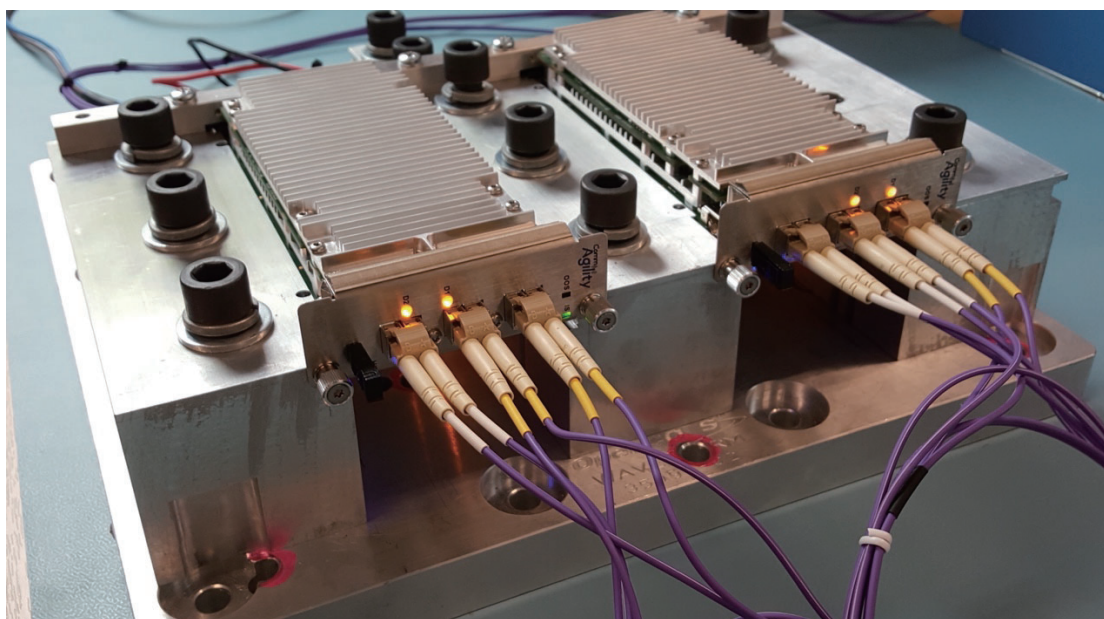
Figure 2: Vibration test jig in the lab, prior to being sent for conformance testing
